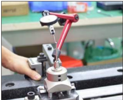
3、检测重复定位精度 Detection of repeated positioning accuracy
