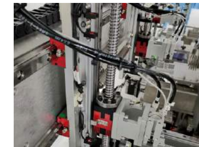
Aligning device for pick - and - place of IC boards
