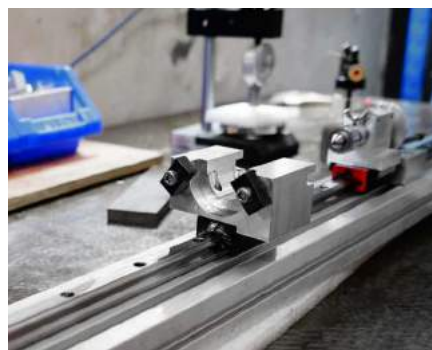
2、检测行走直线绝对精度 Detect the absolute accuracy of the walking straight line
