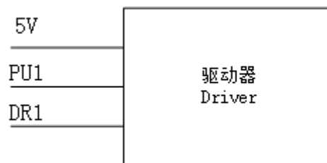
Figure3 Pulse signal wiring
