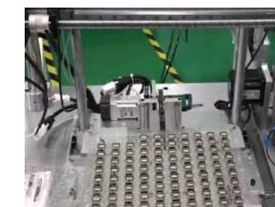
电器元件搬运 Handling of electrical components
